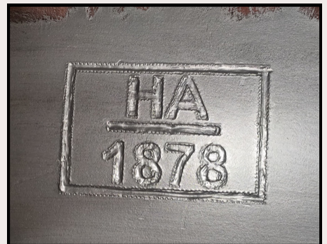
BOILER REGISTRATION NUMBER ENGRAVING
